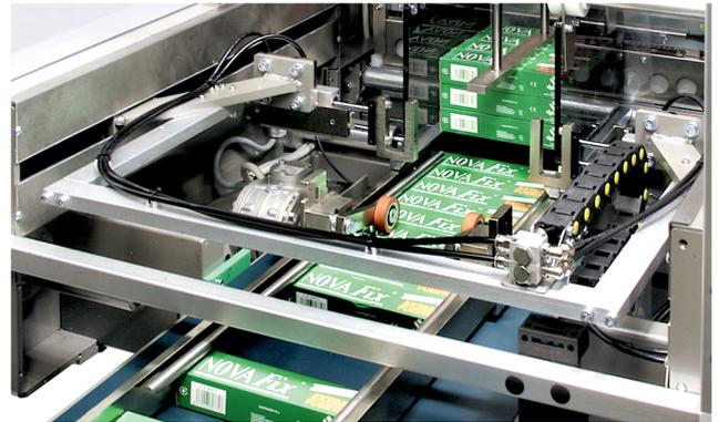
Stacker device for pillow bags with the option of total closing by «spot» lateral sealing station.
