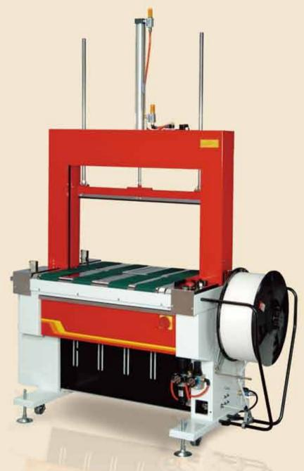
If you are looking for fully automatic strapping machines which offer high reliability and performance, these machines deliver everything you want. All machines are equipped with Electronic Tension Control, Auto Strap Feeding, and Auto Strap Ejector. In this category, we have three models to meet your various needs:
